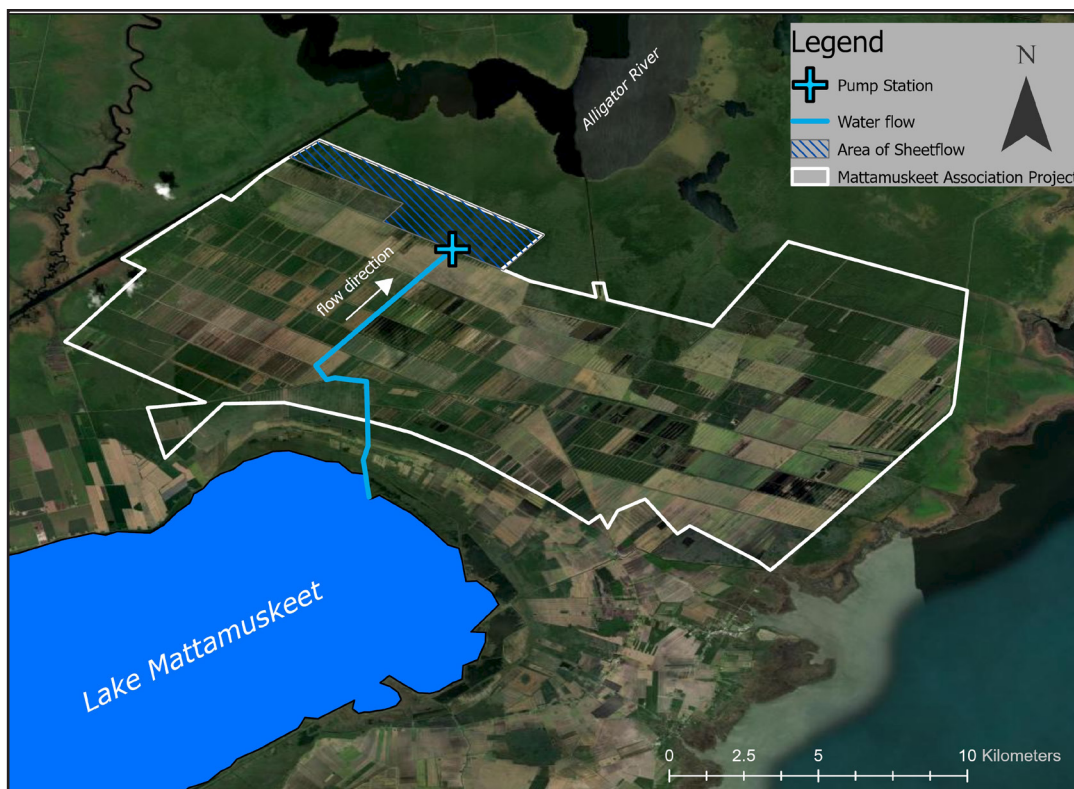
Fig. 4. Concept design for the surface flow wetland project (map image, Esri 2015).
