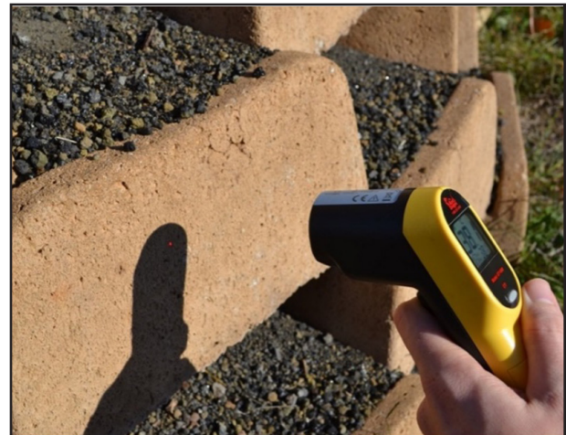
Fig. 4. Surface temperatures of the block were recorded from each aspect with a non-contact infrared thermometer.
