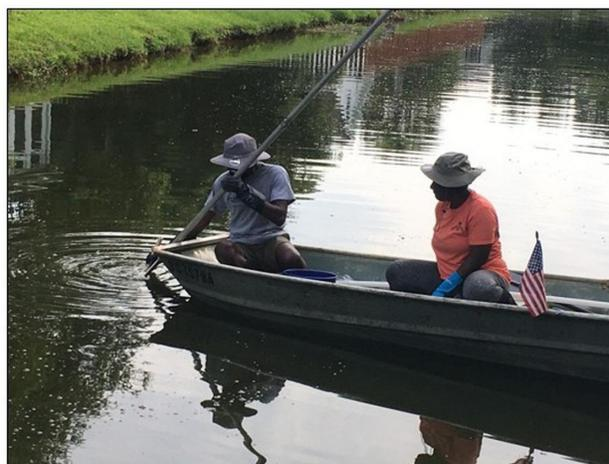
**Study/Project Photographs.** Sampling activity showing the process of using a cup sampler (left) and a sediment borer (right) for water and sediment sample collection.
