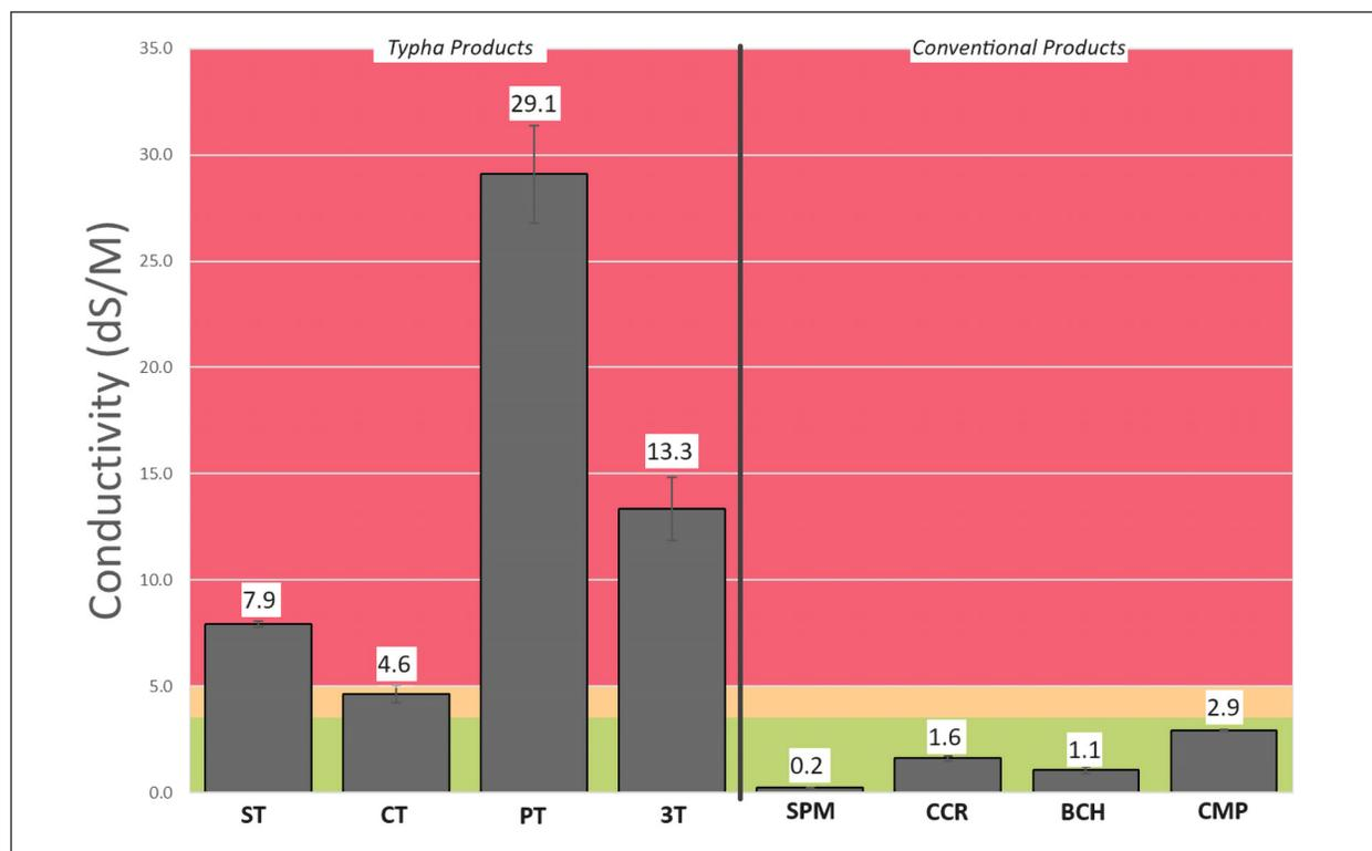
**Fig. 2** Average conductivity  $\pm$  standard deviation for each medium,  $n=3$ . The green, yellow, and red regions represent "Optimum," "High," and "Very High" conductivities, respectively (Warncke 1986). ST=Shredded *Typha*, CT=Composted *Typha*, PT=Pyrolyzed *Typha*, 3T=*Typha* blend, SPM=sphagnum peat moss, CCR=coco coir, BCH=commercial biochar, CMP=commercial potting compost.
