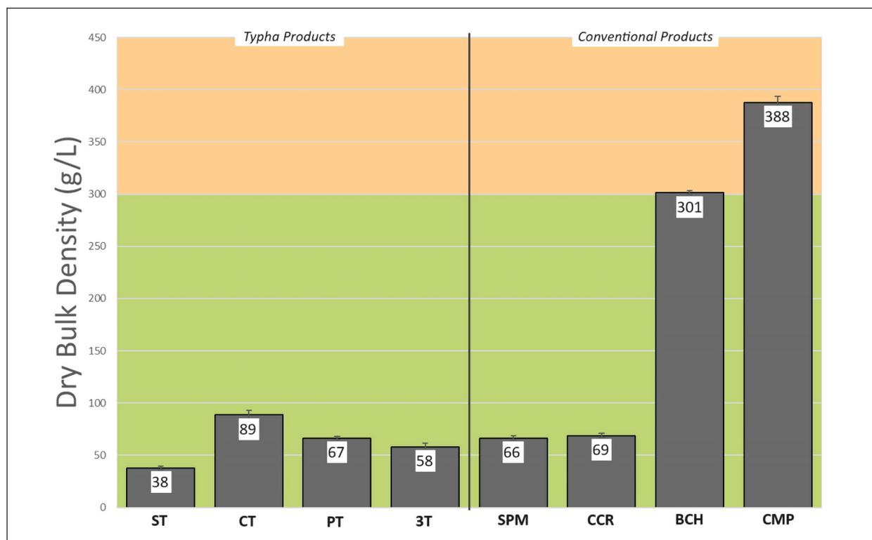
**Fig. 5** Average dry bulk density (DBD)  $\pm$  standard deviation for each medium,  $n=3$ . Green ( $<300$  g/L) and yellow ( $>300$  g/L) regions represent ideal and problematic DBD ranges, respectively (Carlile et al. 2015). ST=Shredded *Typha*, CT=Composted *Typha*, PT=Pyrolyzed *Typha*, 3T=*Typha* blend, SPM=sphagnum peat moss, CCR=coco coir, BCH=commercial biochar, CMP=commercial potting compost.
