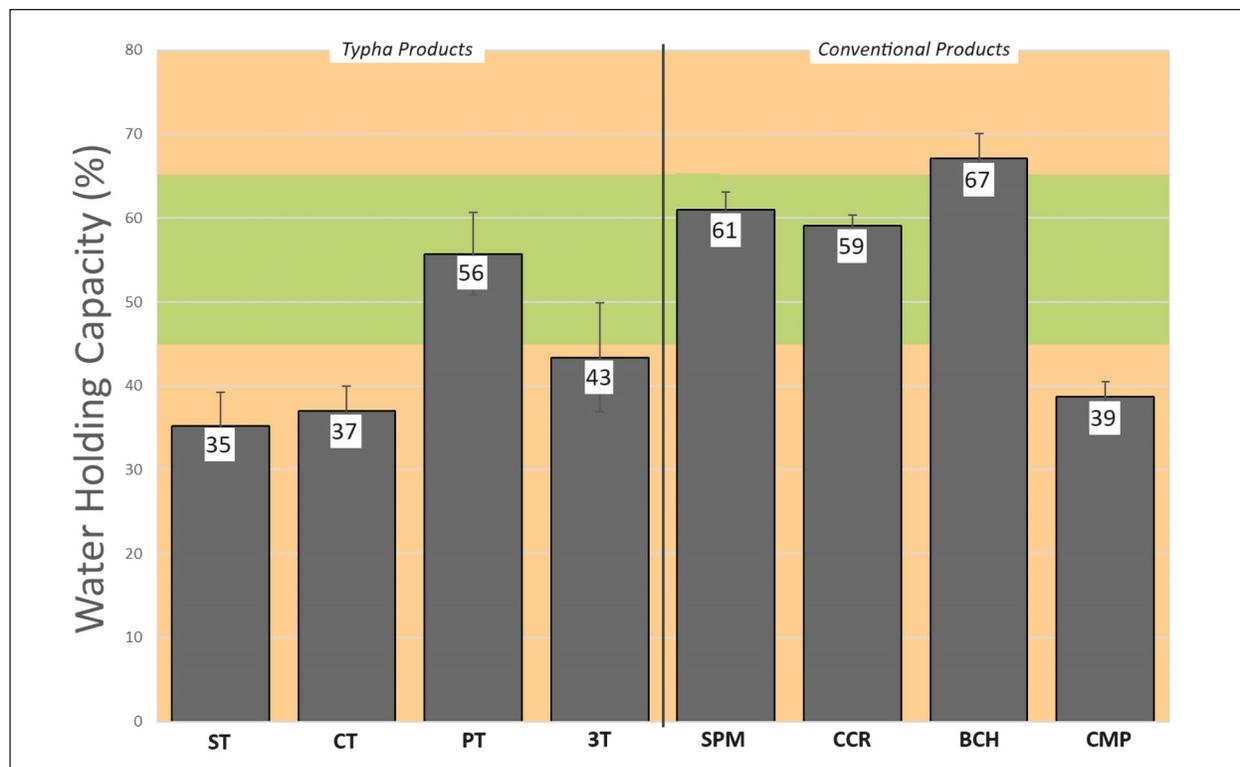
**Fig. 4** Average percentage water holding capacity (WHC)  $\pm$  standard deviation for each medium,  $n=3$ . The green region spanning 45% to 65% represents the optimum WHC for growing media, while the yellow regions outside this range represent suboptimal WHC (Bilderback et al. 2005). ST=Shredded *Typha*, CT=Composted *Typha*, PT=Pyrolyzed *Typha*, 3T=*Typha* blend, SPM=sphagnum peat moss, CCR=coco coir, BCH=commercial biochar, CMP=commercial potting compost.
